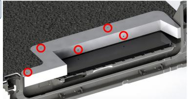
"After placing the floor in place along with the steel sill above it, mark and drill holes of 0.25 inches at the five locations highlighted in red."
