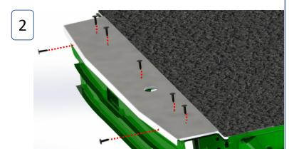
"Insert push-in rivets in the holes drilled"
