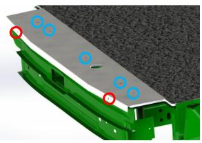
"After placing the floor in place along with the steel sill above it, mark and drill holes of 0.25 inches at the five/seven locations highlighted." (Please refer to the note below)
