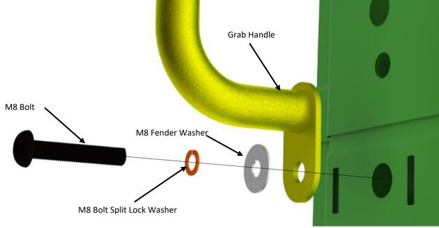
"Hardware to be used at the Lower Fastening Point"
