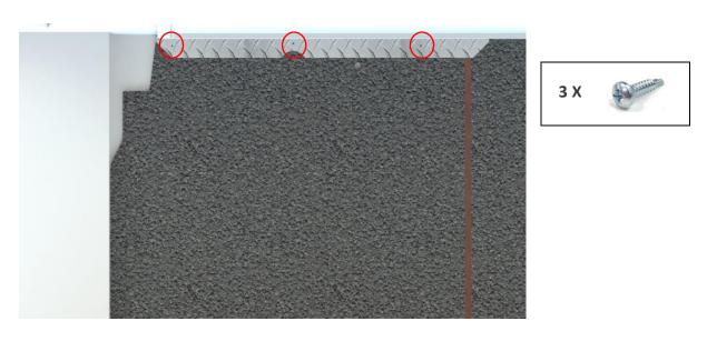
Figure 5 "Positioning and Fixing of the Side Sill"
