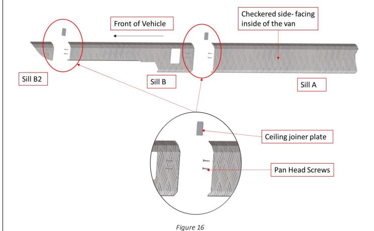
**Step 4:** Fasten assembled sills in the Van.
