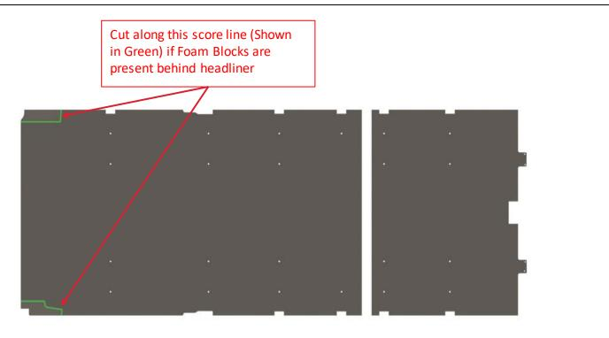
**Step 1:** Install Ceiling Piece A, as shown below.
