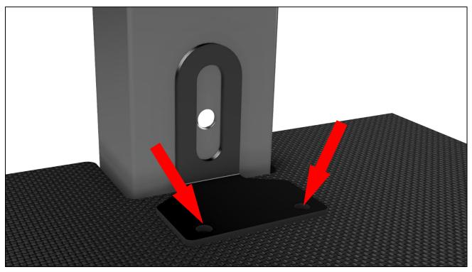
**Step 3**: Drill two 23/64" holes through the flooring, using the markings from step 2, and screw the provided M6 threaded inserts into the top side of the flooring, using the 6mm Allen key.
