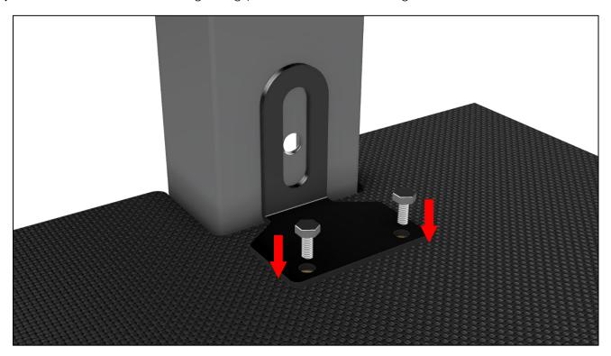
**Step 5**: Attach Bracket to vehicle frame using the OEM bolt from Step 1.
