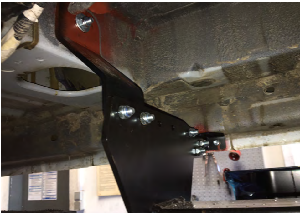
FIGURE 7: MOUNTING POINTS X3 FORD TRANSIT
