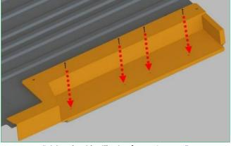
"Fixing the side sill using four #10 screws"
