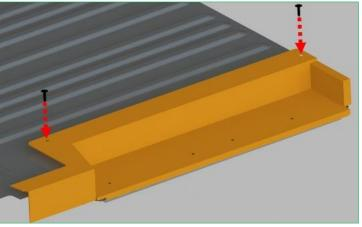
"Installing two push-in rivets in the side sill"
