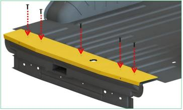
"Installing five push-in rivets to secure the rear sill"
