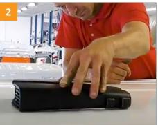
2. Place the foam gasket underneath the VanFan and push the tubes through the holes with the grille at the front. *Note:* the foam gasket should be fitted at all times! The foam gasket is available separately in a range of thicknesses: ask our specialists for advice on the correct thickness to use.
