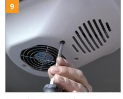
Secure the VanFan module cover plate using the three screws provided.
