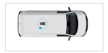
If you have 1 fan, place it as close as possible to the centre point of the roof which can be determined by measuring from the bulkhead to the tailgate or rear doors.
