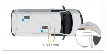
If you have 2 fans, place them diagonally so that they are evenly spaced. Divide the space into 3 equal parts lengthwise (measured from the bulkhead to the tailgate or rear doors) and place the VanFan 1/3 from the front and 1/3 from the rear and widthwise half-way along the half-diagonal.
